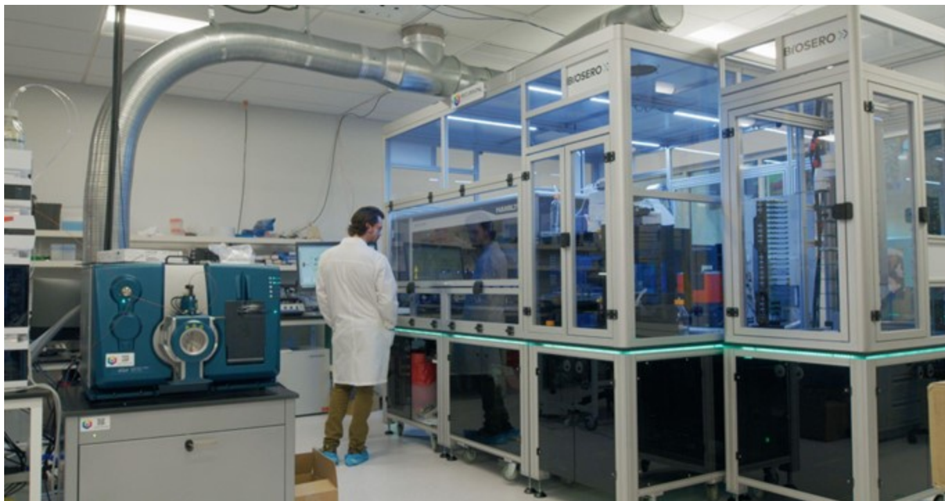
Figure 28. Recursion’s automated DMPK system allows for automated assay execution across plasma protein binding, microsomal stability and cell permeability studies at scale to advance programs while generating state-of-the-art training data for ML and AI algorithm development. The system has been designed to allow for future potential addition of additional modules into the automated workflow such as addition in vitro absorption, distribution, metabolism, excretion, and toxicity (ADMET) testing.
