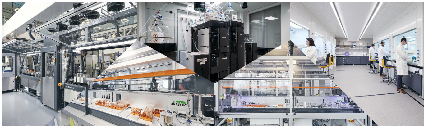
Figure 24. Recursion's automated chemistry wet lab, a modular system for chemical synthesis preparation, execution, analysis, work-up, and purification.
