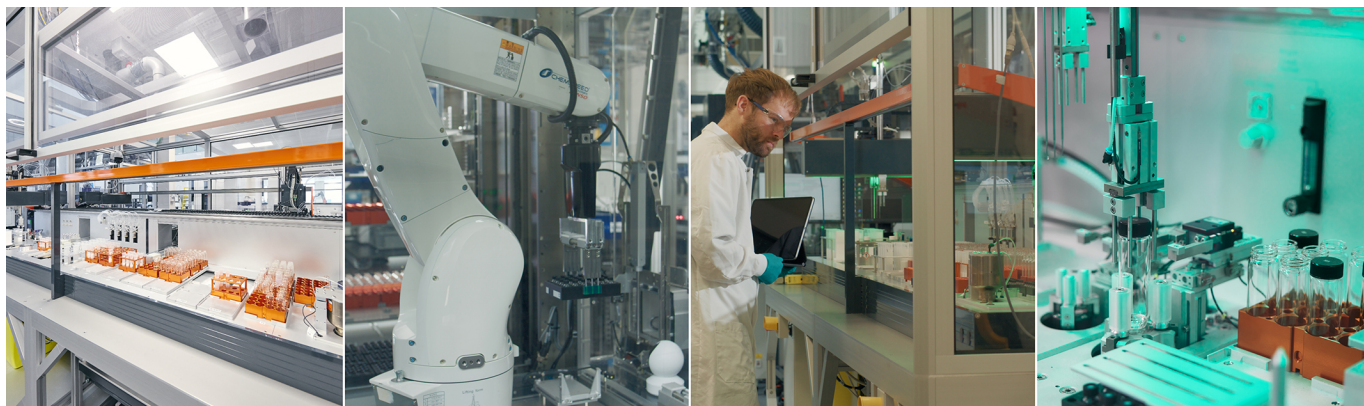
Figure 37. Recursion's automated chemistry wet lab, a modular system for chemical synthesis preparation, execution, analysis, work-up, and purification.
