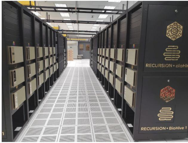
**Figure 19. We believe BioHive-1 is one of the most powerful supercomputers dedicated wholly to drug discovery for a single company.** BioHive-1 consists of 40 NVIDIA DGX A100 640GB nodes which further expands our capability to rapidly improve ML models.
