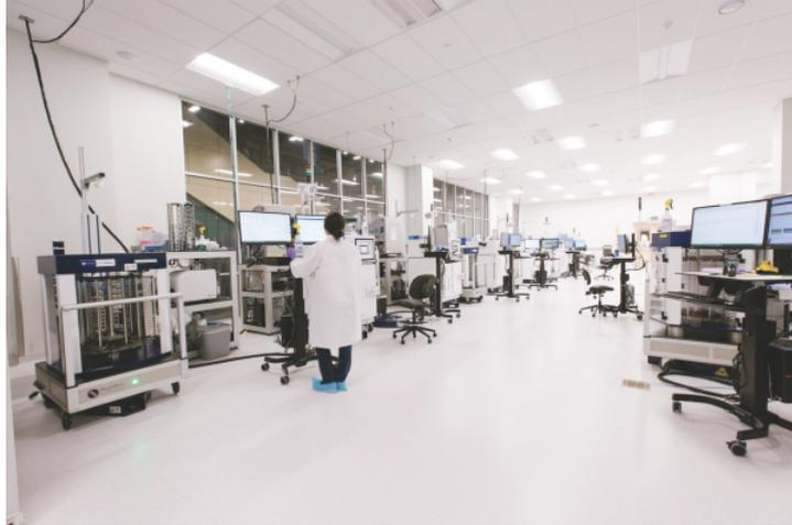
**Figure 15.** Our high-throughput automation platform looks more like a sophisticated manufacturing facility than a biology R&D laboratory. Our platform can execute up to 2.2 million experiments each week with high-quality to enable downstream analyses.
